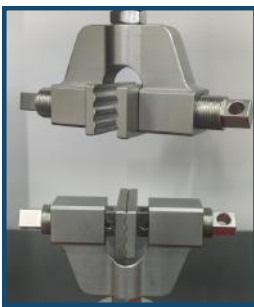
JG 25017 Vice Grip 2kN (450lbf) for Fabric and leather
