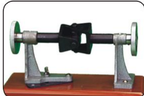
(6) Crossed shaft universal coupling
